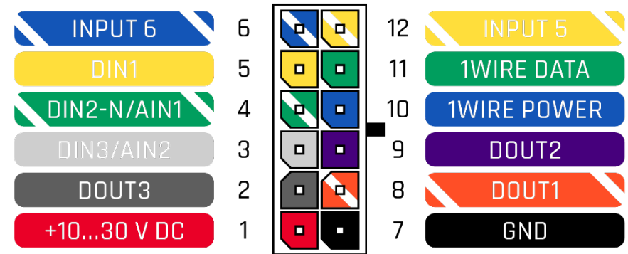
Figure 2 FMM130 2x6 socket pinout
